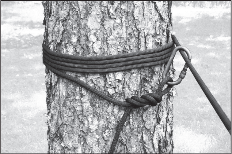
Figure 9-4. Tensionless natural anchor
